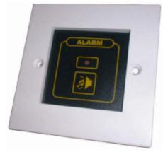
Connects to the Remote Relay inside the Pressmatic to indicate an issue with the equipment at a remote location. Usually installed in a Security, Management, Janitorial, Caretakers or Custodians office to indicate a problem with the main equipment (that is usually located elsewhere in a basement or plant room or otherwise sometimes rarely accessible location). Requires 110-240vAC or 12-24vAC/DC Power. Made to BS5733.
